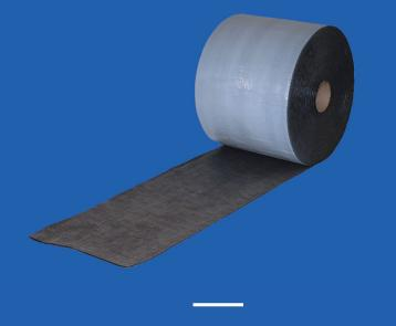
"650 Sheet Membrane is a strong, pliable, 60-mil, post-concrete pour self-adhesive waterproofing membrane and vapor retarder, virtually eliminating water and vapor transmission through concrete walls & slabs. 650 Sheet Membrane is designed for use numerous architectural applications but for highway applications is most commonly used for box culvert waterproofing.
