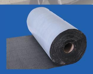
"Cold Flex™ SA Membrane is a high strength waterproofing and crack reduction membrane installed as a "peel and stick" material. Cold Flex™ SA has a top layer of high strength fabric, with a thick layer of rubberized asphalt adhesive sealant to provide stress relief and waterproofing. The stress relief layer is reinforced with a second layer of high strength fabric.
