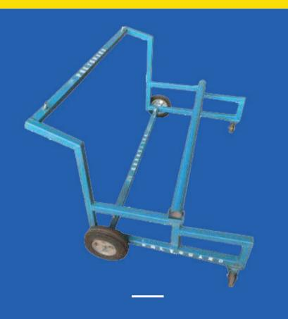
The Polyguard Membrane Installation Cart, is designed to assist installation of our highway and bridge deck membranes in a quick and efficient manner. The carts is adjustable for widths from 12" – 48". The top rail holds the roll of membrane while the bottom rail applies tension while the membrane is applied. Typically a two person job with one person directing the cart over the bridge deck or joint/crack, and the other gathering the release liner.
