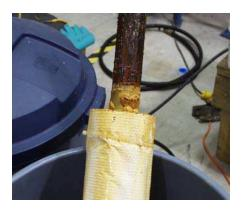
At 81 days, this sample was removed. This pipe was one of those with mill scale as received. It had no corrosion on the treated area.
