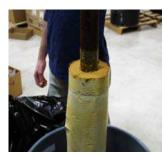
At 31 days, a pipe was removed and cleaned. A difference in corrosion is already apparent. Note the transition area above the tag; at this area the insulation cover slipped down a couple of inches during the test. When this was discovered, all pipes remaining in the saltwater bath had the insulation secured and the test proceeded.
