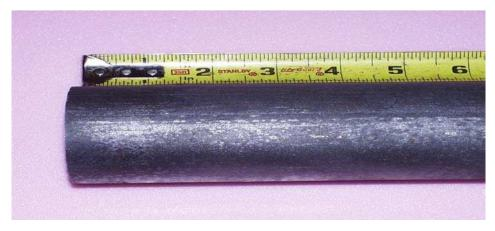
Both bead blasted pipe and mill scale as received were used in the test. A close-up of bead blasted pipe is above.
