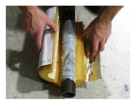
The RG reactive gel was spread over the pipe and the fiberglass insulation placed over the bottom portion. The untreated portion acted as a control.
