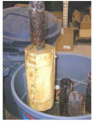
At 365 days, this sample was removed. Inspection showed no corrosion on the treated area.
