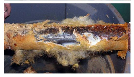
After two years, the insulation had begun to rot, but there was almost no corrosion on the treated area under the insulation.
