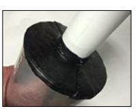
TYPICAL PHYSICAL PROPERTIES and GENERAL INFORMATION **PROPERTY VALUE** RAW MATERIAL BASE **BUTYL RUBBER** CONE PENETRATION @ 77° F, 100G 7.6mm COLOR **BLACK** THICKNESS 1.4" WIDE 20 MIL THICKNESS 12" WIDE 40 MIL SHELF LIFE ONE YEAR FORM & PACKAGING TAPE ROLLS PHYSICAL STATE FLEXIBLE SOLID **ODOR NEUTRAL** ADHESION TO STEEL 87 oz. per inch TENSILE STRENGTH 9 lbs/in SERVICE TEMP (MAX) 200°F
