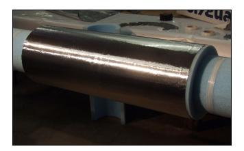
ZeroPerm® vapor barrier acrylic tapes are required for use with Polyguard Products ZeroPerm vapor barrier membrane to seal butt joints and longitudinal joints and for use on valves and fittings. Made from the same material as the ZeroPerm vapor barrier, the tapes maintain an absolute "zero perm" barrier that provides maximum protection for all types of insulations used in below ambient, sub-freezing and cryogenic applications on duct, pipe, or vessel systems
