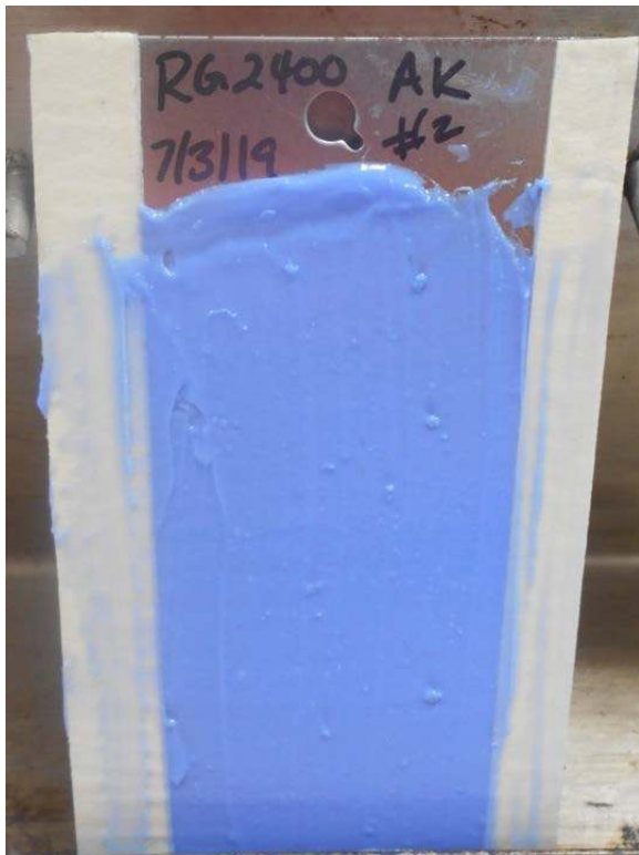
Sample 2 pre heat exposure
