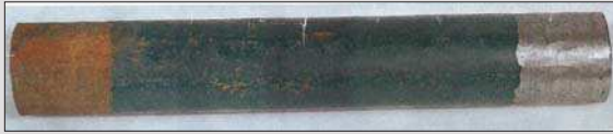
Figure 10: Pipe Treated with SPHT on One End, then Exposed to the Florida Coastal Elements for One Month
