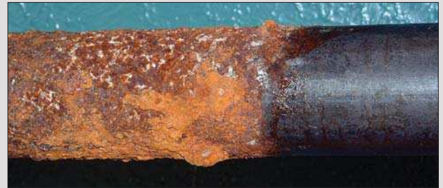
Figure 14: Two-Year Test Pipe after RG Is Cleaned off
