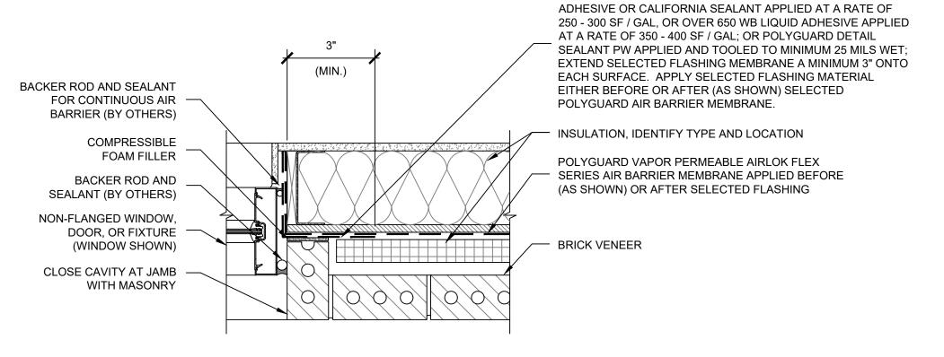
04 AFFP PLAN @ FRAMED BACKING WALL / MASONRY VENEER - NON-FLANGED WINDOW, DOOR, OR FIXTURE - JAMB
