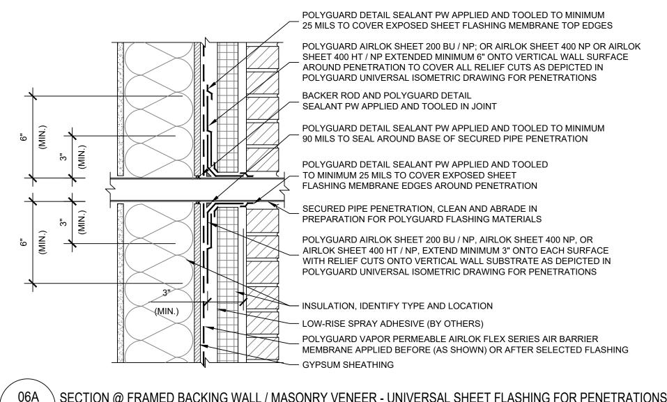
SECTION @ FRAMED BACKING WALL / MASONRY VENEER - UNIVERSAL SHEET FLASHING FOR PENETRATIONS
