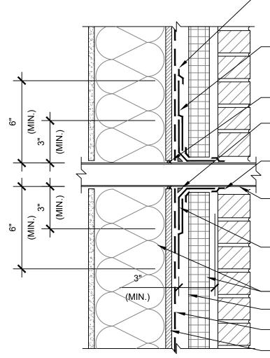
POLYGUARD DETAIL SEALANT PW APPLIED AND TOOLED TO MINIMUM 25 MILS TO COVER EXPOSED SHEET FLASHING MEMBRANE TOP EDGES
