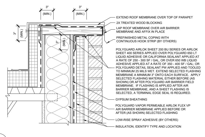
08 AFFP SECTION @ FRAMED BACKING WALL / MASONRY VENEER - PARAPET
