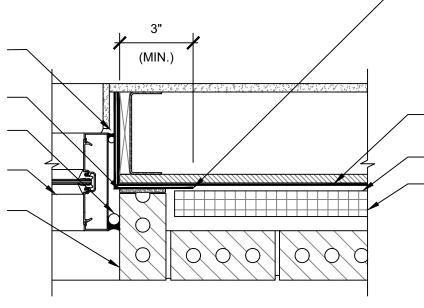
POLYGUARD AIRLOK SHEET 200 BU SERIES OR AIRLOK SHEET 400 SERIES APPLIED OVER POLYGUARD 650 LT LIQUID ADHESIVE OR CALIFORNIA SEALANT APPLIED AT A RATE OF 250 - 300 SF / GAL, OR OVER 650 WB LIQUID ADHESIVE APPLIED AT A RATE OF 350 - 400 SF / GAL; OR POLYGUARD DETAIL SEALANT PW APPLIED AND TOOLED TO MINIMUM 25 MILS WET. EXTEND SELECTED FLASHING A MINIMUM 3" ONTO EACH SURFACE. APPLY SELECTED FLASHING EITHER BEFORE OR AFTER (AS SHOWN) SELECTED POLYGUARD AIR BARRIER FIELD MEMBRANE.
