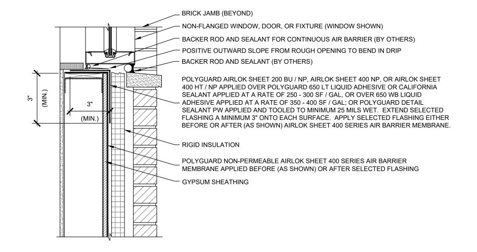
ackslash SECTION @ FRAMED BACKING WALL / MASONRY VENEER - NON-FLANGED WINDOW, DOOR, OR FIXTURE SILL
