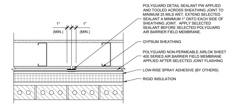
PLAN @ FRAMED BACKING WALL / MASONRY VENEER - SUBSTRATE JOINT
