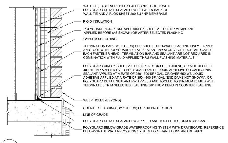
SECTION @ FRAMED BACKING WALL / MASONRY VENEER - WALL BASE
