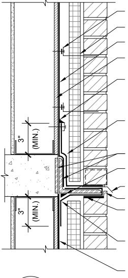
WALL TIE, FASTENER HOLE SEALED AND TOOLED WITH POLYGUARD DETAIL SEALANT PW BETWEEN BACK OF WALL TIE AND AIRLOK SHEET 200 BU / NP MEMBRANE
