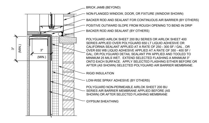
SECTION @ FRAMED BACKING WALL / MASONRY VENEER - NON-FLANGED WINDOW, DOOR, OR FIXTURE SILL
