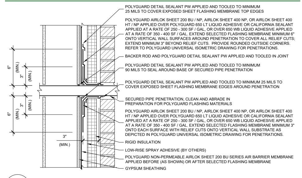
06A SECTION @ FRAMED BACKING WALL / MASONRY VENEER - UNIVERSAL SHEET FLASHING FOR PENETRATIONS
