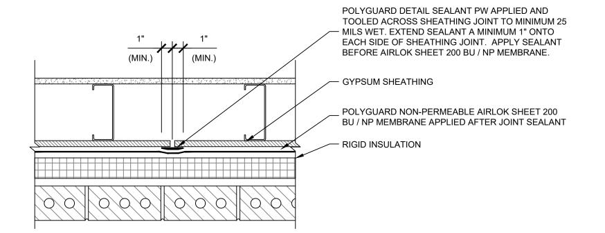
ackslash PLAN @ FRAMED BACKING WALL / MASONRY VENEER - SUBSTRATE JOINT
