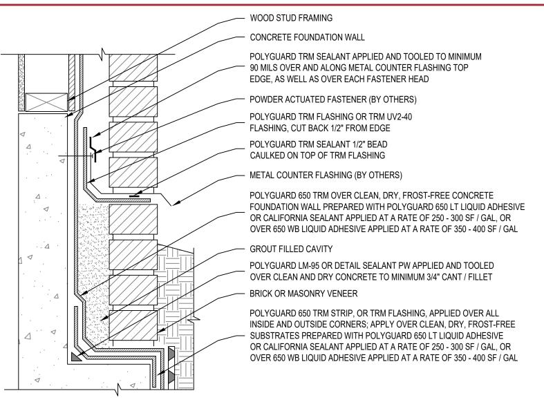
SECTION @ TRM FLASHING - THRU-WALL FLASHING INSTALLATION
