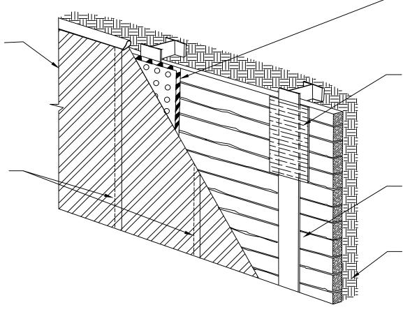
POLYGUARD POLYFLOW 15 / 15P SHEET MOLDED DRAIN FABRIC FACING RETENTION SYSTEM
