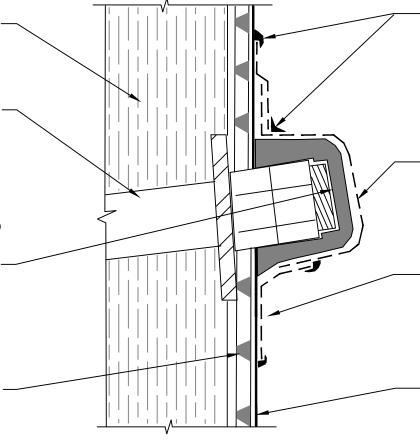
POLYGUARD DETAIL SEALANT PW OR POLYGUARD LM-95 APPLIED OVER TERMINATION OF POLYGUARD FABRIC TAPE AND ONTO POLYGUARD BLINDSIDE MEMBRANE - PREPARE FABRIC WITH POLYGUARD 650 LT LIQUID ADHESIVE OR POLYGUARD CALIFORNIA SEALANT AT A RATE OF 50 - 75 SF/GAL
