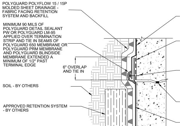
POLYGUARD 650 MEMBRANE 0R POLYGUARD PRM MEMBRANE APPLIED TO CLEAN, DRY, FROST FREE SUBSTRATE PREPARED WITH POLYGUARD 650 LT LIQUID ADHESIVE OR POLYGUARD CALIFORNIA SEALANT AT A RATE OF 250 - 300 SF/GAL AND ONTO EXISTING POLYGUARD BLINDSIDE MEMBRANE MINIMUM OF 6"
