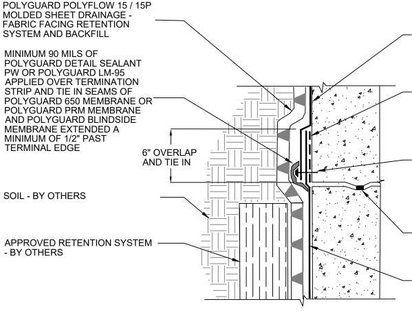
POLYGUARD 650 MEMBRANE 0R POLYGUARD PRM MEMBRANE APPLIED TO CLEAN, DRY, FROST FREE SUBSTRATE PREPARED WITH POLYGUARD 650 LT LIQUID ADHESIVE OR POLYGUARD CALIFORNIA SEALANT AT A RATE OF 250 - 300 SF/GAL AND ONTO EXISTING POLYGUARD BLINDSIDE MEMBRANE MINIMUM OF 6"
