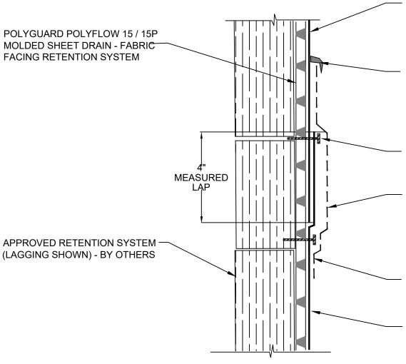
POLYGUARD BLINDSIDE MEMBRANE FABRIC FACING CONCRETE POUR OR SHOTCRETE WHEN NOT IN WATER TABLE - IF IN WATER TABLE CONSULT POLYGUARD - APPLIED BEHIND EXISTING BLINDSIDE SHEET A MAXMIUM 4"
