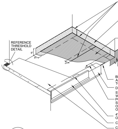
SEAL TOP EDGE OF POLYGUARD 105 FLASHING AND ALL SEAMS OF POLYGUARD BALCONY SHEET MEMBRANE SERIES WATERPROOFING WITH POLYGUARD DETAIL SEALANT PW OR POLYGUARD LM-95 APPLIED AND TOOLED - REFER TO BW3
