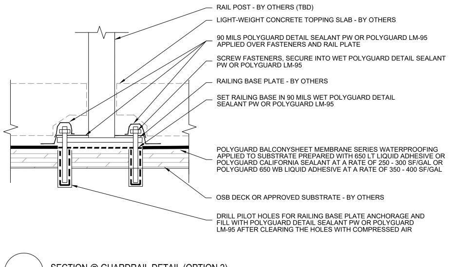
BW11 SECTION @ GUARDRAIL DETAIL (OPTION 2)
