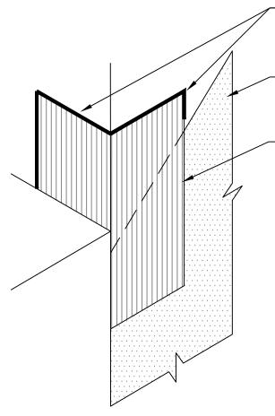
SEAL TOP EDGE OF POLYGUARD BALCONY SHEET MEMBRANE SERIES WATERPROOFING FLASHING WITH POLYGUARD DETAIL SEALANT PW OR LM-95 APPLIED AND TOOLED DIRECTLY TO RAW SHEATHING SUBSTRATE TO MINIMUM 60 MILS THICK; EXTEND MINIMUM 1" ON EACH SIDE OF JOINT, AND HOLD BACK POLYGUARD DETAIL SEALANT PW OR LM-95 FROM ANY CONTACT WITH EXISTING MECHANICALLY ATTACHED SHEET AIR BARRIER BY MINIMUM 1/2-INCH GAP.
