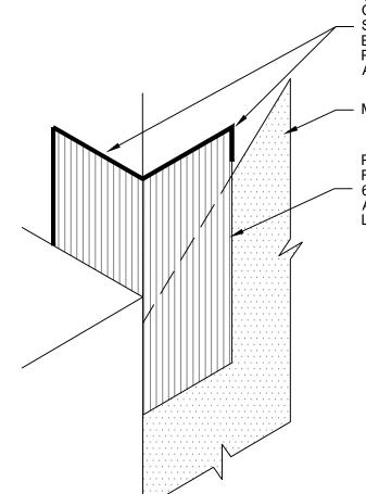
SEAL TOP EDGE OF POLYGUARD BALCONY SHEET MEMBRANE SERIES WATERPROOFING FLASHING WITH POLYGUARD DETAIL SEALANT PW OR LM-95 APPLIED AND TOOLED DIRECTLY TO RAW SHEATHING SUBSTRATE TO MINIMUM 60 MILS THICK; EXTEND MINIMUM 1" ON EACH SIDE OF JOINT, AND HOLD BACK POLYGUARD DETAIL SEALANT PW OR LM-95 FROM ANY CONTACT WITH EXISTING MECHANICALLY ATTACHED SHEET AIR BARRIER BY MINIMUM 1/2-INCH GAP.
