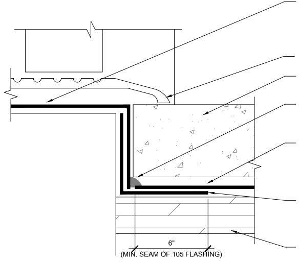
APPLY A STRIP OF POLYGUARD BALCONY SHEET MEMBRANE SERIES WATERPROOFING OVER POLYGUARD 650 LT LIQUID ADHESIVE OR POLYGUARD CALIFORNIA SEALANT APPLIED AT A RATE OF 250 -300 SF / GAL OR POLYGUARD 650 WB LIQUID ADHESIVE APPLIED AT A RATE OF 350 -400 SF / GAL EXTENDING UP 2" ONTO DOOR JAMB TO CREATE A THRESHOLD PAN.
