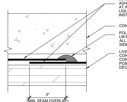
POLYGUARD BALCONY SHEET MEMBRANE SERIES WATERPROOFING OVER POLYGUARD 650 LT LIQUID ADHESIVE OR POLYGUARD CALIFORNIA SEALANT APPLIED AT A RATE OF 250 - 300 SF / GAL OR POLYGUARD 650 WB LIQUID ADHESIVE APPLIED AT A RATE OF 350 - 400 SF / GAL, INSTALL IN SHINGLE MANNER WITH MINIMUM 3" OVERLAP
