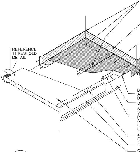
SEAL TOP EDGE OF POLYGUARD 105 FLASHING AND ALL SEAMS OF POLYGUARD BALCONY SHEET MEMBRANE SERIES WATERPROOFING WITH POLYGUARD DETAIL SEALANT PW OR POLYGUARD LM-95 APPLIED AND TOOLED TO MINIMUM 60-MILS, EXTEND MINIMUM 1" ON EACH SIDE OF JOINT
