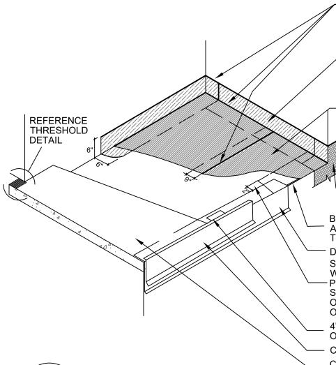
SEAL TOP EDGE OF POLYGUARD 105 FLASHING AND ALL SEAMS OF POLYGUARD BALCONY SHEET MEMBRANE SERIES WATERPROOFING WITH POLYGUARD DETAIL SEALANT PW OR POLYGUARD LM-95 APPLIED AND TOOLED - REFER TO BW 6
