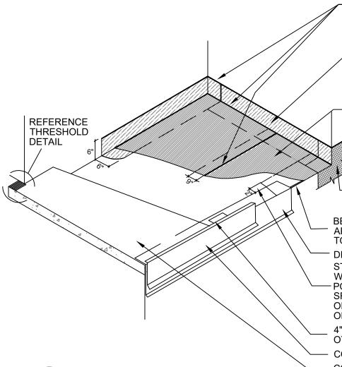
SEAL TOP EDGE OF POLYGUARD 105 FLASHING AND ALL SEAMS OF POLYGUARD BALCONY SHEET MEMBRANE SERIES WATERPROOFING WITH POLYGUARD DETAIL SEALANT PW OR POLYGUARD LM-95 APPLIED AND TOOLED - REFER TO BW 6
