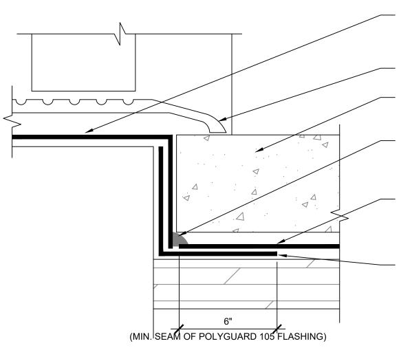
APPLY A STRIP OF POLYGUARD BALCONY SHEET MEMBRANE SERIES WATERPROOFING OVER POLYGUARD 650 LT LIQUID ADHESIVE OR POLYGAURD CALIFORNIA SEALANT APPLIED AT A RATE OF 250 -300 SF / GAL OR POLYGUARD 650 WB LIQUID ADHESIVE APPLIED AT A RATE OF 350 -400 SF / GAL EXTENDING UP 2" ONTO DOOR JAMB
