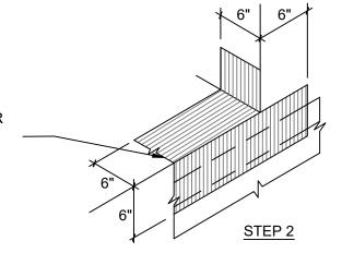
POLYGUARD DETAIL TAPE FLASHING (PIECE #2) OVER CLEAN AND DRY SUBSTRATES PREPARED WITH POLYGUARD 650 LT LIQUID ADHESIVE OR POLYGUARD CALIFORNIA SEALANT AT A RATE OF 250 - 300 SF / GAL, OR POLYGUARD 650 WB LIQUID ADHESIVE AT A RATE OF 350 - 400 SF / GAL
