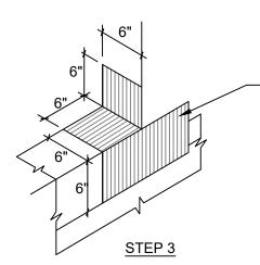
POLYGUARD DETAIL TAPE FLASHING (PIECE #1) OVER CLEAN AND DRY SUBSTRATES PREPARED WITH POLYGUARD 650 LT LIQUID ADHESIVE OR POLYGUARD CALIFORNIA SEALANT AT A RATE OF 250 - 300 SF / GAL, OR POLYGUARD 650 WB LIQUID ADHESIVE APPLIED AT A RATE OF 350 - 400 SF / GAL
