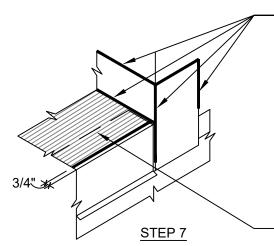
POLYGUARD 105 FLASHING APPLIED TO SUBSTRATES PREPARED WITH POLYGUARD 650 LT LIQUID ADHESIVE OR POLYGUARD CALIFORNIA SEALANT AT A RATE OF 250 - 300 SF / GAL, OR POLYGUARD 650 WB LIQUID ADHESIVE AT A RATE OF 350 - 400 SF / GAL
