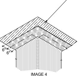
POLYGUARD FABRIC TAPE, EXTEND 6" TO EACH SIDE OF THE POLYGUARD CRM MEMBRANE END LAP
