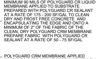
POLYGUARD CRM MEMBRANE APPLIED FABRIC TOWARD CONCRETE POUR WITH END ONTO A MINIMUM OF 2" OF CONCRETE AND WET POLYGUARD CR LIQUID MEMBRANE
