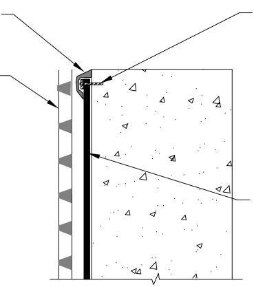
1/8" X 1" METAL TERMINATION BAR FASTENED AT 8" SPACING AND 2" FROM EACH END - BY OTHERS
