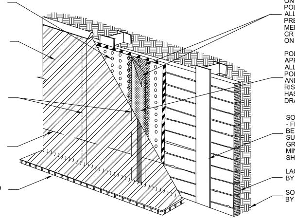
SPRAY A 12" WIDE AREA OF LOW RISE SPRAY ADHESIVE ONTO DRAINBOARD AND ONTO POLYGUARD CR SEAM TAPE ALLOW TO FLASH OFF AND PRESS POLYGUARD CRM MEMBRANE AND POLYGUARD CR SEAM TAPE INTO ADHESIVE ON POLYGUARD POLYFLOW 15
