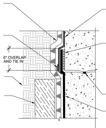
POLYGUARD ULTRA CRM MEMBRANE APPLIED TO CLEAN, DRY, FROST FREE SUBSTRATE PREPARED WITH POLYGUARD 650 LT LIQUID ADHESIVE OR POLYGUARD CALIFORNIA SEALANT AT A RATE OF 250 - 300 SF/GAL AND ONTO EXISTING POLYGUARD CRM MEMBRANE MINIMUM OF 6"
