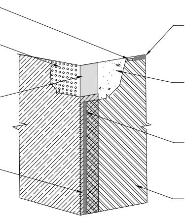
MINIMUM 90 MILS OF POLYGUARD CR LIQUID MEMBRANE APPLIED TO THE TERMINAL EDGE OF TERMINATION STRIP COVERING FASTENERS AND EXTENDING 1/2" ABOVE AND BELOW TERMINATION STRIP - PREPARE SURFACE WITH POLYGUARD CR SEALANT AT A RATE OF 175 - 200 SF/GAL PRIOR TO POLYGUARD CR LIQUID MEMBRANE
