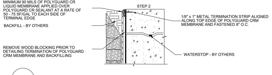
CRV16 SECTION @ TOP OF WALL TERMINATION MECHANICALLY FASTENED
