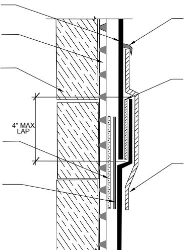
COVERING BEAD OF POLYGUARD DETAIL SEALANT PW OR POLYGUARD LM-95 APPLIED TO FABRIC OF POLYGUARD BLINDSIDE MEMBRANE. PREPARE FABRIC BEING COVERED WITH POLYGUARD 650 LT LIQUID ADHESIVE OR POLYGUARD CALIFORNIA SEALANT AT A RATE OF 50 - 75 SF/GAL
