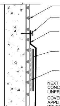
POLYGUARD POLYFLOW 15 MOLDED DRAINAGE BOARD - FABRIC FACING RETENTION SYSTEM
