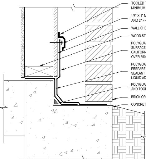
POLYGUARD DETAIL SEALANT PW OR TRM SEALANT APPLIED AND TOOLED TO MINIMUM 90 MILS OVER TERMINATION BAR; EXTEND MINIMUM 1/8" BEYOND PERIMETER OF EACH FASTENER HEAD
