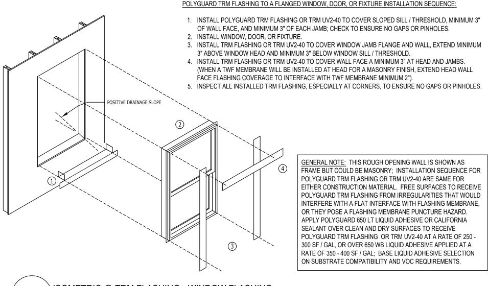
ISOMETRIC @ TRM FLASHING - WINDOW FLASHING
